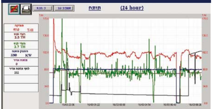
Figure 3: Nesher control panel showing a typical shift before the Silo-Flow™ installation. Green line showing gypsum feed and red line showing cement production. Note 5 gypsum stoppages with the 5th leading to cement production stoppage
